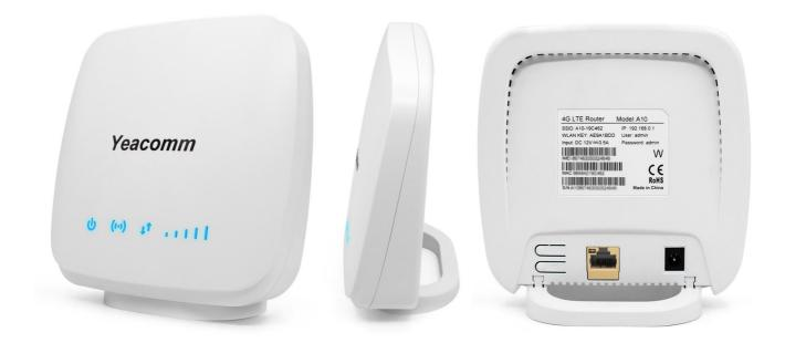
YF-A10 is a high-performance wireless communication 4G LTE CPE. It is mainly used for data transmission services, equipment monitoring, wireless routing and other functions. YF- A10 adopts high-performance processor, which can process protocol and large amount of data at high speed. It can be used with a variety of 4G CAT4 module, providing 802.11b/g/n Wi-Fi access.
